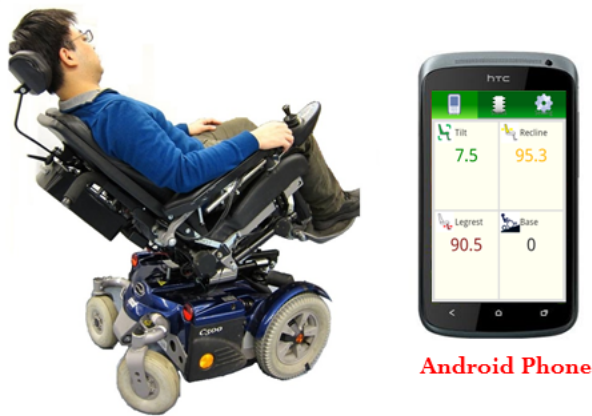
Figure 4. The user interface shows the seat tilt, backrest recline, legrest elevation and wheelchair base inclination information.
