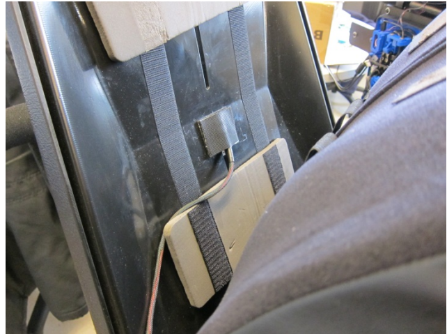
Figure 6. The accelerometer can be quickly taped onto the wheelchair with hook and loop fastener.
